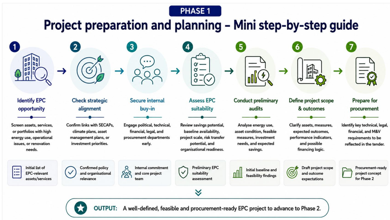
Figure 4. Simplified roadmap for Phase 1 EPC project preparation and planning
